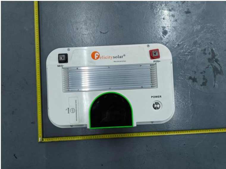
Battery: FLA12300, 12.8V, 300Ah, 3.75kWh
